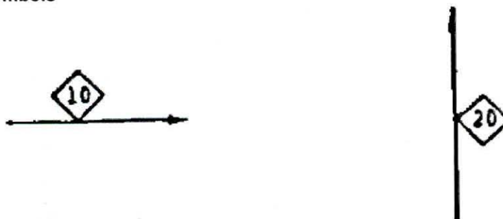
PIPELINE SYMBOLS Fig. 1.1 (a)
