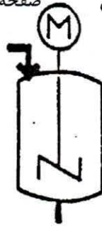
VESSEL WITH AGITATOR DRIVEN BY ELECTRIC MOTOR
